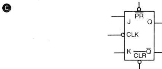
Fig. 8-19. Pin-out, state table, and logic symbol of the LS76A J-K flip-flop.
